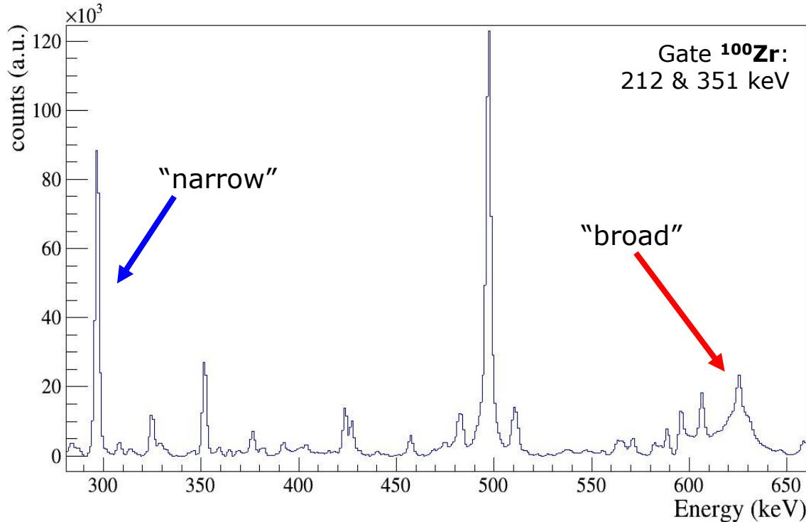
Doppler broadening of the gamma-ray peak following the de-excitation of the slowing down fission fragment (active target)
