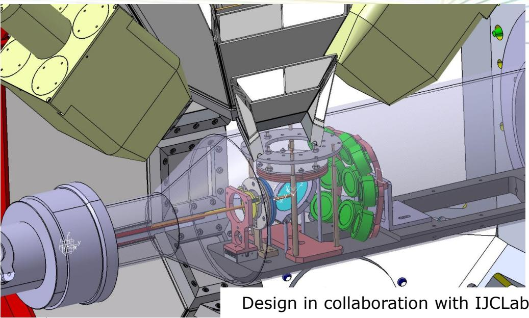
Design and simulation of the fission fragment detection system which allows to have a mass resolution of 3-5 amu
