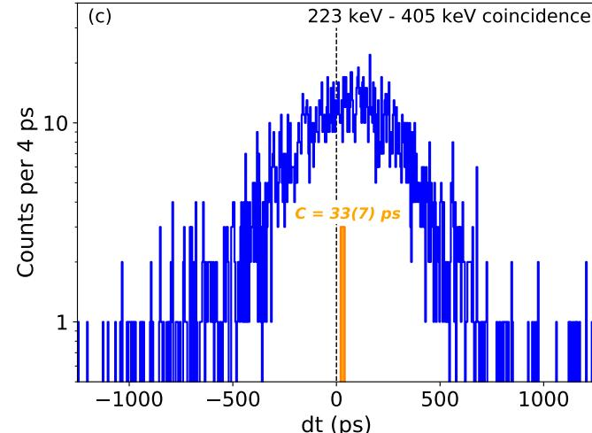
$$\tau_{4_1^+} = C_{cor}^D(223 \text{ keV}, 405 \text{ keV}) - PRC(223 \text{ keV}, 405 \text{ keV})$$
