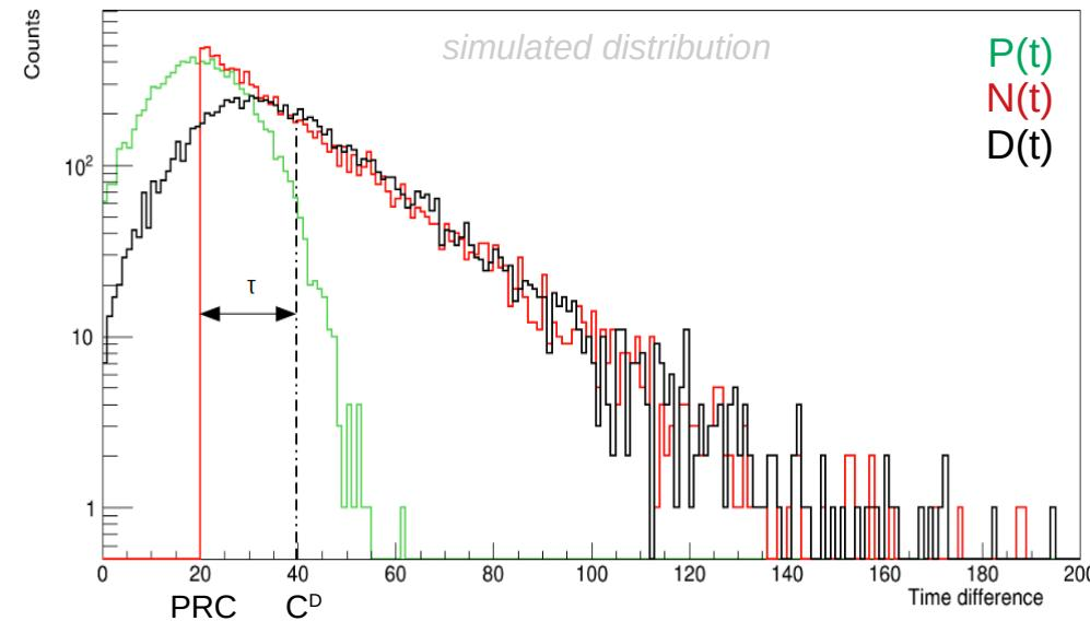
$$C^D(E_{\text{feeder}}, E_{\text{decay}}) = \tau + PRC(E_{\text{feeder}}, E_{\text{decay}})$$
