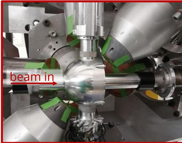
**SONIC:** 12 (telescope) silicon particle detectors
