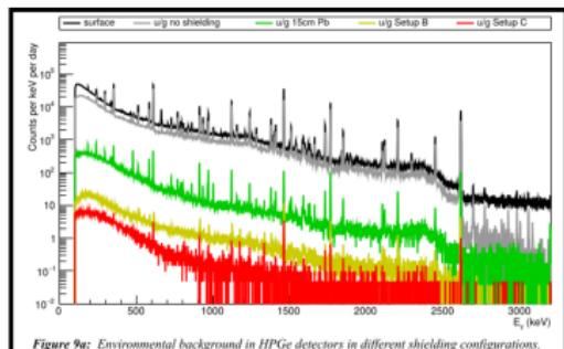
Figure 9a: Environmental background in HPGe detectors in different shielding configurations.
