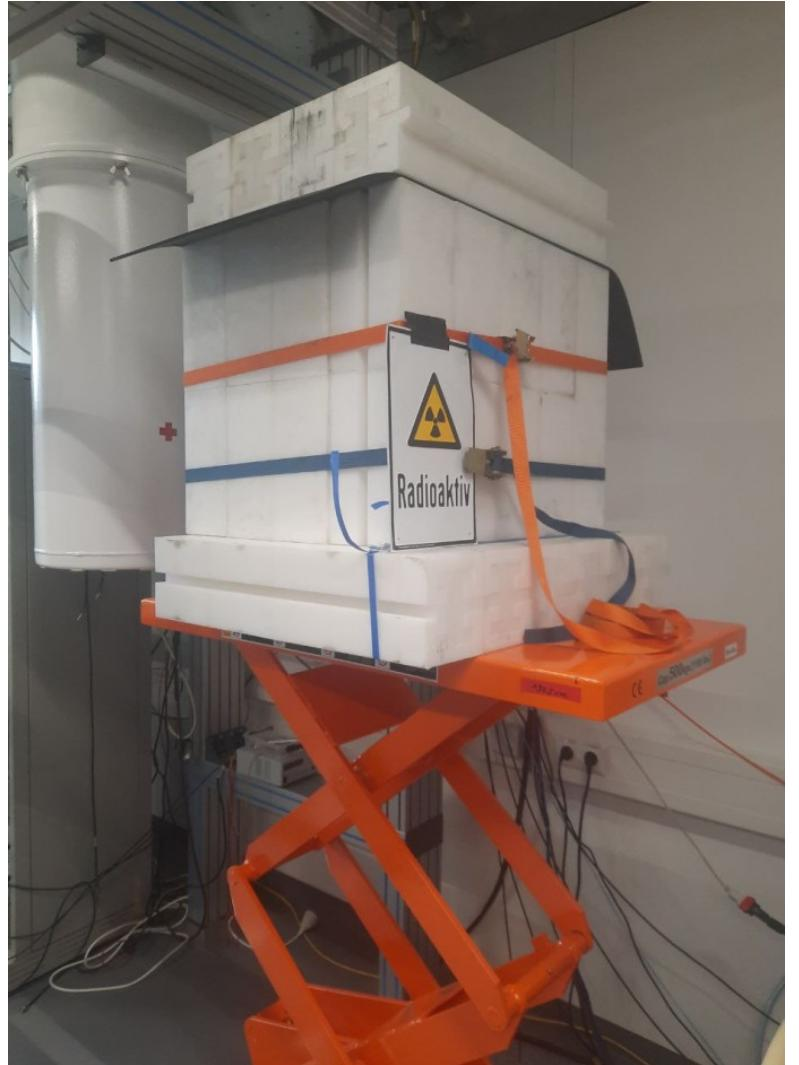
**Thermal neutrons** produced with a 3.7 MBq
