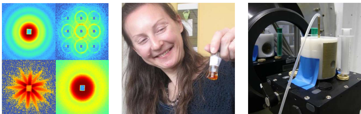
Left: Christmas card 2012 designed by Isabelle showing first results from D33. Center: Isabelle Right: Stopped-flow with temperature controlled cell holder designed and donated from the University of Cologne at D33.
