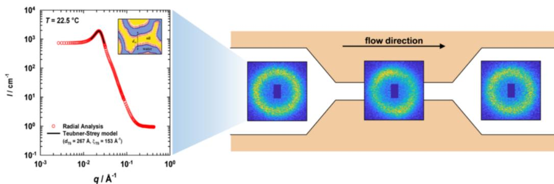
Figure 1: (Left) SANS curve of a bicontinuously structured microemulsion, fitted with the Teubner-Strey model [6] (Right) 2D-scattering patterns of the same system under flow before, inside, and after the constriction of a Microfluidic SANS chip.
