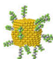
Figure 1: Example of a gold nanoparticle simulated by DISCUS. The particle is shaped as cubeoctahedron and decorated by fluorinated thiooctane molecules [4].
