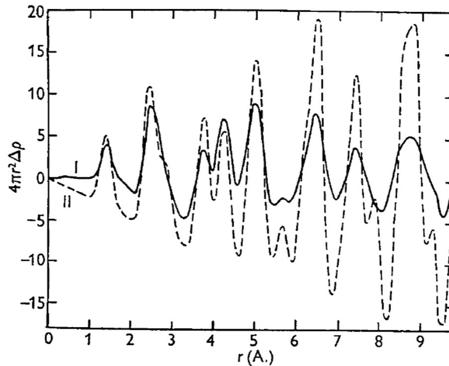
Fig. 6. Curve I, the atomic distribution function obtained after multiplying the corrected intensity curve by  $\exp(-0.4s^2)$ . Curve II, the function which would be given by a single infinite graphite layer under the same conditions.
