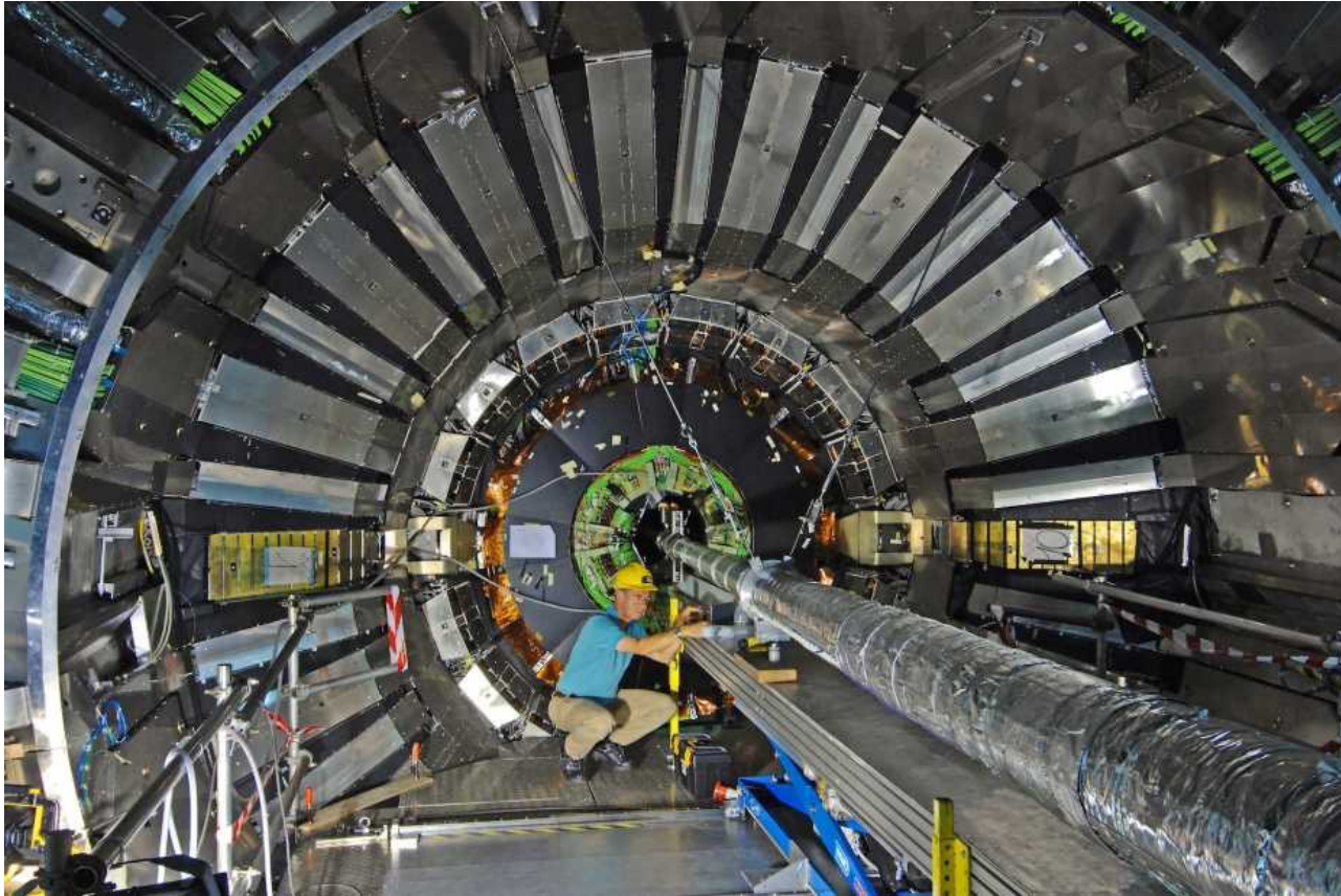
Roland Horisberger fitting one of the final pieces of the CMS pixel detector at LHC (10 September 2008). (Photo: ETH Zurich / H.R. Bramaz; source ETH Zürich)
