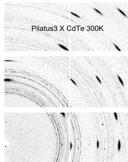
Superconducting filament,  $\varnothing 50 \mu\text{m}$ , measured at 50 keV, with exposure time of 100ms with a Perkin Elmer XRD 1621 flat panel detector (left) and with the Dectris Pilatus3 X CdTe 300K prototype
