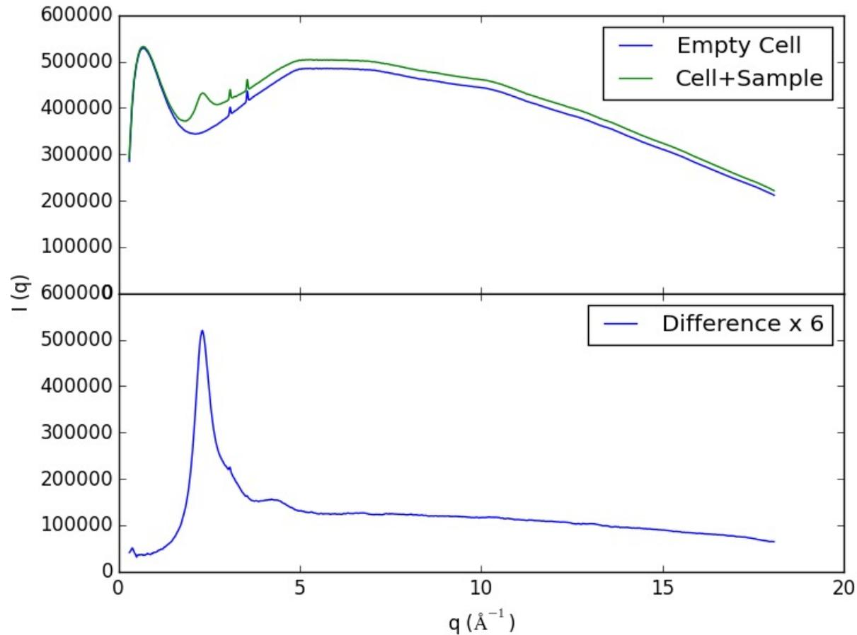
Signal from the material of interest is a small fraction of the total signal
