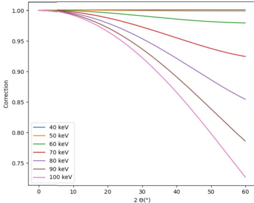
The precise correction would consider the path length in adjacent pixels, but this effect is swamped by others
