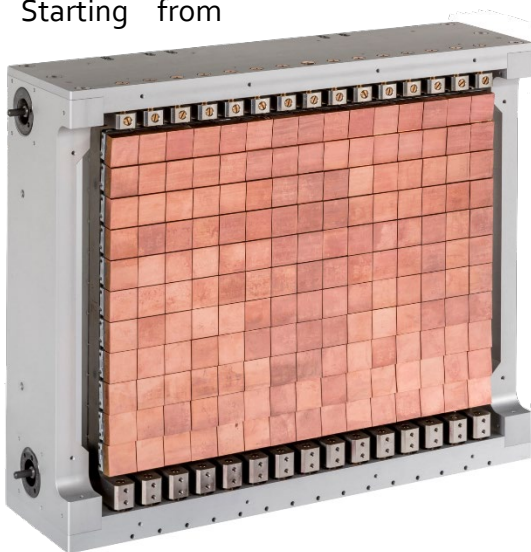
Figure 1: The new double focusing Cu(220) monochromator for the thermal time-of-flight PANTHER. The monochromator comprises 165 Copper pieces for a total active area of 660 cm 2 .
