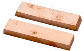
Crystal cutting by spark erosion
