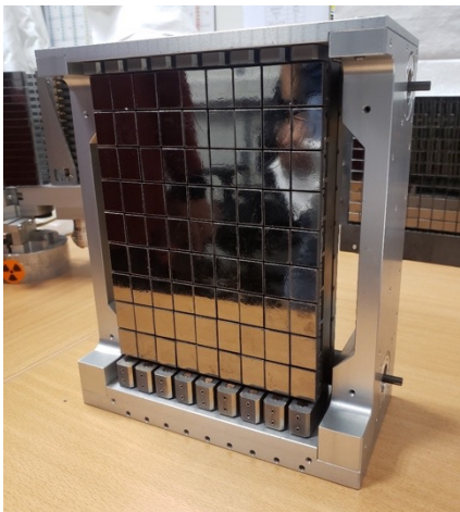
HOPG Monochromator 81 crystals (19 x 15 x 2 mm 3 )
