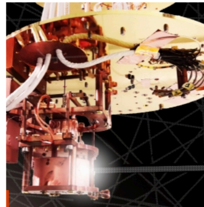
R&D cryostat used for the development of Ricochet bolometers / Image IPNL
