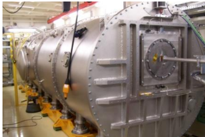
Large chamber under vacuum housing the X-rays detector
