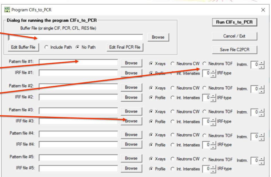
Program to refine powder diffraction patterns (X-rays and FAULTS neutrons) of crystal systems with any type of coherent planar defect. Based on DIFFaX and CrysFML
