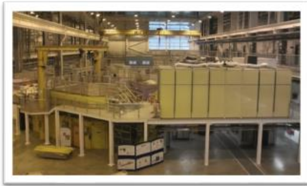
Near and InterMediate Range Order Diffractometer (NIMROD) with Q-range of 0.01 to 50 \text{\AA}^{-1}
