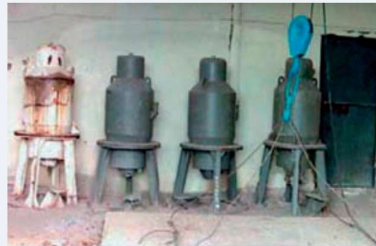
Kolos Facility (USSR) Cs137 Max: 129TBq
