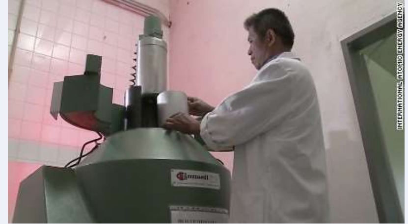
Gammcell 220 (Canada) Co60 Max: 999TBq Up to 48 pencil sources
