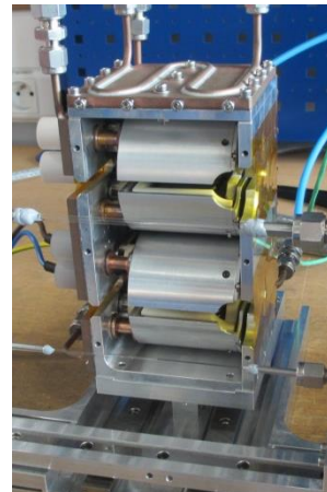
(b) Capillary cells 20 bar, RT – 1000°C
