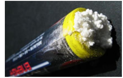
Crystallized Electrolyte of a Leaked Alkaline Cell (Turelio BY CC 3.0)
